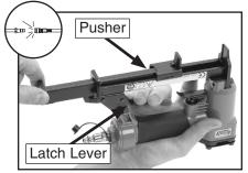
Figure 5. Opening stapler magazine.
